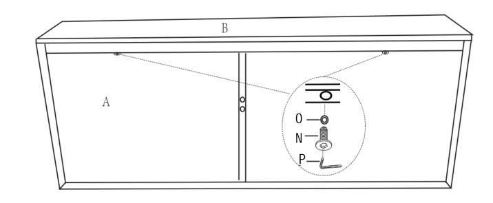
Connect the seat frame to the front panel with screws and washers
